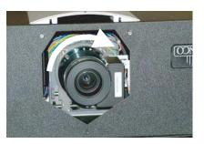
10. Secure the lens assembly to the projector flange with the three Allen screws that you loosened in Step 6.
